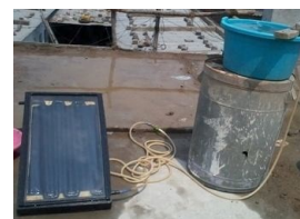
Figure 8: Experimental Setup of flat plate collector
